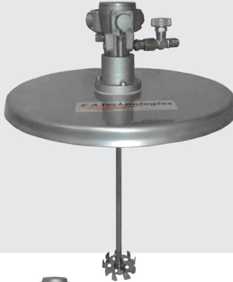
The TechLine economy mixers are for the professional wanting a good mixer at a great price. All of these units are constructed of steel and have stainless steel shafts. The 54-400, 54-410 and 54-450 units have plastic blades, all other models have stainless steel blades. The air motors are piston type motors for longer life.
